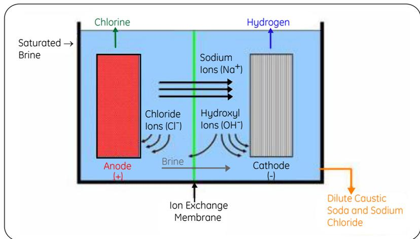
**Figure 2.** Chlor Alkali Production
