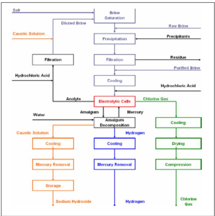
Figure 1. Chlor alkali process
