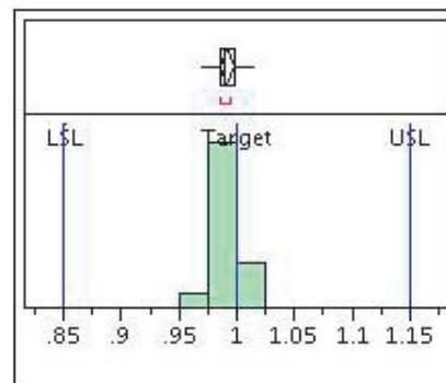
**Figure 5e.** Calculated response efficiencies, and specification limits for Sievers 900, serial number 531.
