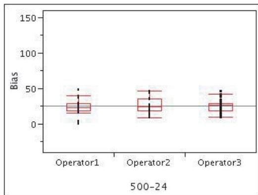
**Figure 2a.** Box plots of the bias report for Operator from Sievers 500 RL, serial number 24.
