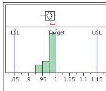
**Figure 5c.** Calculated response efficiencies, and specification limits for Sievers 900, serial number 405.
