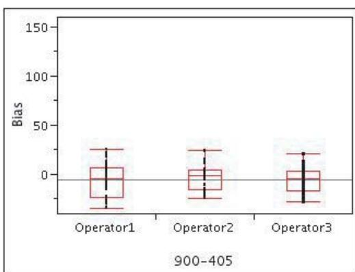
**Figure 2c.** Box plots of the bias report for operator from Sievers 900, serial number 405.
