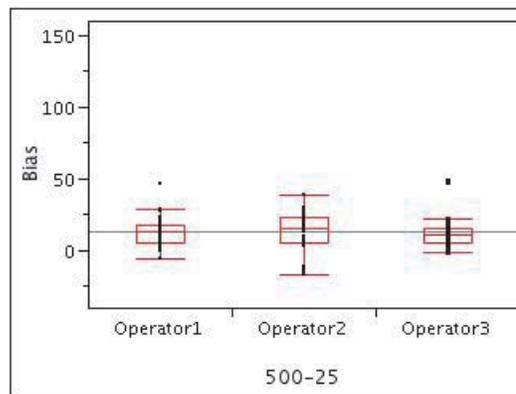
**Figure 2b.** Box plots of the bias report for operator from Sievers 500 RL, serial number 25.
