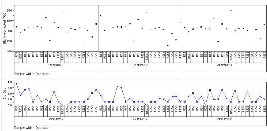
Figure 1b. Variability and standard deviation plots from Sievers 500 RL, serial number 24.
