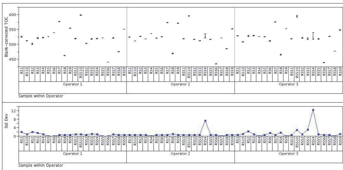
**Figure 1a.** Variability and standard deviation plots from Sievers 500 RL, serial number 21.
