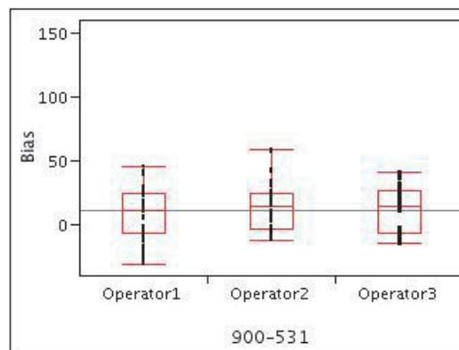
**Figure 2e.** Box plots of the bias report for operator from Sievers 900, serial number 531.
