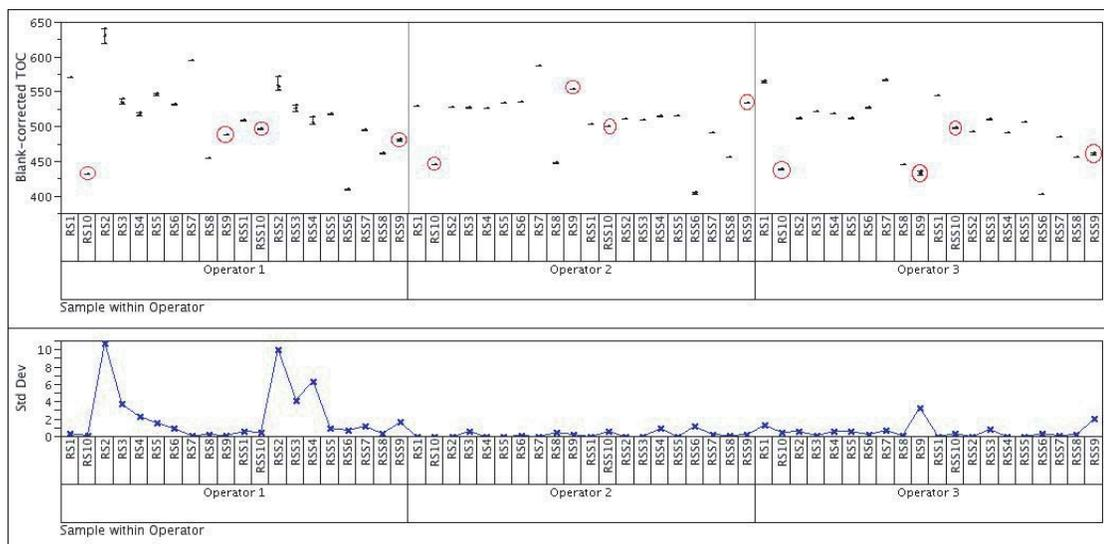
Figure 1d. Variability and standard deviation plots from Thornton 5000TOC. Circled data were excluded from study due to instrument malfunction.
