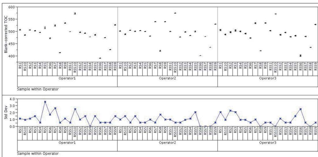
Figure 1c. Variability and standard deviation plots from Sievers 900, serial number 405
