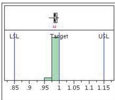
**Figure 5b.** Calculated response efficiencies, and specification limits for Sievers 500 RL, serial number 25.
