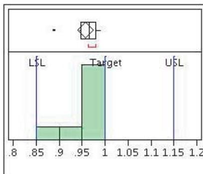
**Figure 5d.** Calculated response efficiencies, and specification limits for Thornton 5000TOC.
