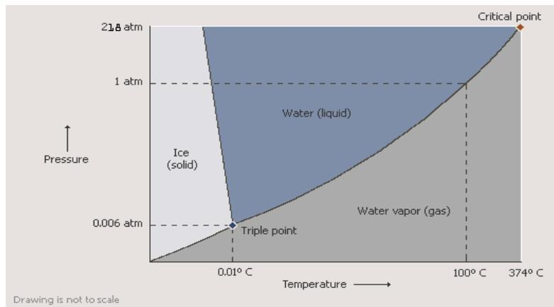
Figure 1. Phase diagram of water
