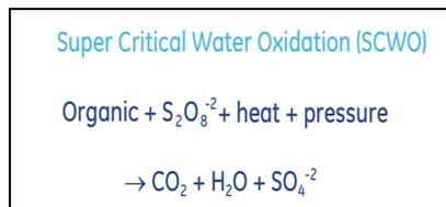
Figure 2. Supercritical Water Oxidation
