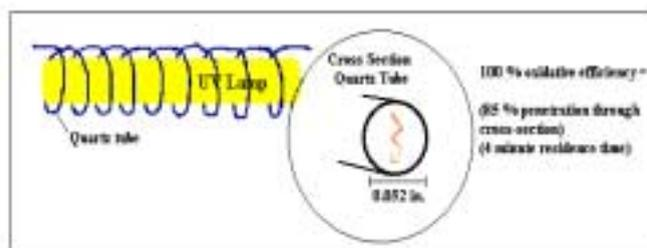
Figure III. Sievers Continuous Flow Oxidation Cell
