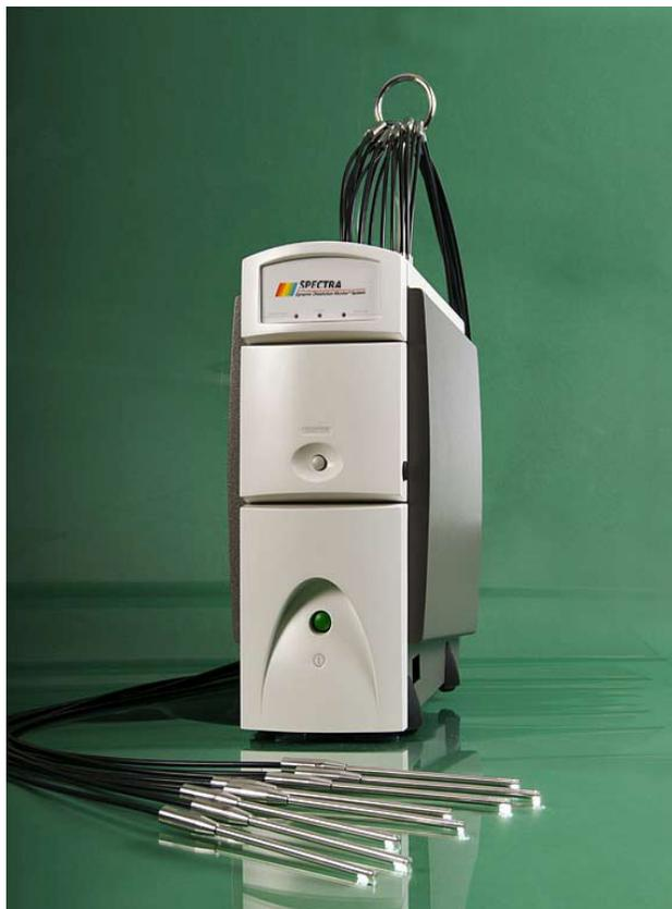
The Spectra measures the API (active pharmaceutical ingredient) concentration in real-time using fiber optic probes immersed in the dissolution vessels. While the traditional approach of removing liquid samples from the vessels is prone to plugging and requires frequent maintenance, the Spectra collects the entire UV-vis spectrum (200-720 nm) directly from the solution and displays concentration data in real time.
